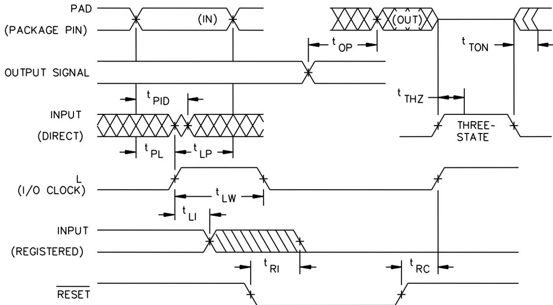
FIGURE 3. Timing diagrams and switching characteristics – continued.
