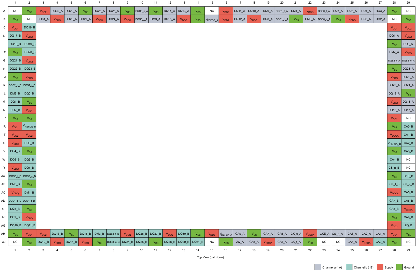
Figure 2: 216-Ball FBGA – 2 x 4Gb Die
