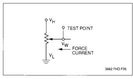
Notes: (1) Absolute Linearity is utilized to determine actual wiper voltage versus expected voltage =  $(V_{w(n)}(actual) - V_{w(n)}(expected)) = \pm 1$  Ml Maximum. (2) 1 Ml = Minimum Increment =  $R_{TOT}/99$ .
