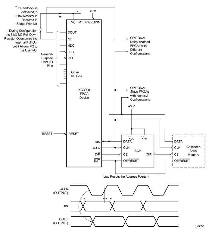
**Figure 2:** Master Serial Mode. The one-time-programmable Serial Configuration PROM supports automatic loading of configuration programs. Multiple devices can be cascaded to support additional FPGA. An early D/P inhibits the PROM data output one CCLK cycle before the FPGA I/Os become active.
