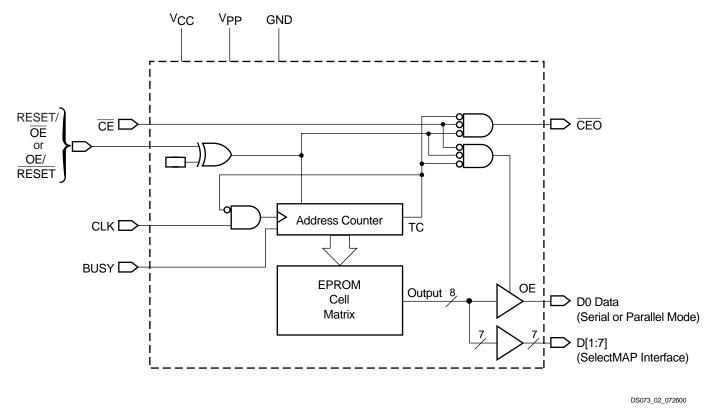
Figure 1: Simplified Block Diagram for XQR17V16 (does not show programming circuit)
