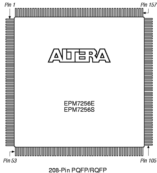
Figure 24. 208-Pin Package Pin-Out Diagram
