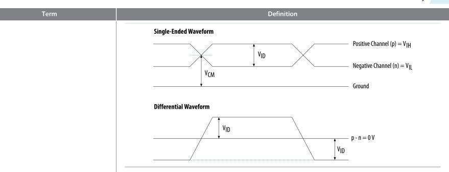
Transmitter Output Waveforms
