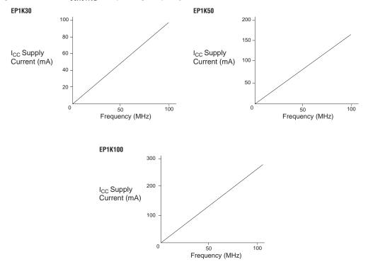
Figure 31. ACEX 1K I<sub>CCACTIVE</sub> vs. Operating Frequency
