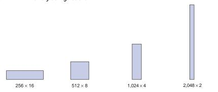
Larger blocks of RAM are created by combining multiple EABs. For example, two  $256\times16$  RAM blocks can be combined to form a  $256\times32$  block, and two  $512\times8$  RAM blocks can be combined to form a  $512\times16$  block. Figure 6 shows examples of multiple EAB combination.
