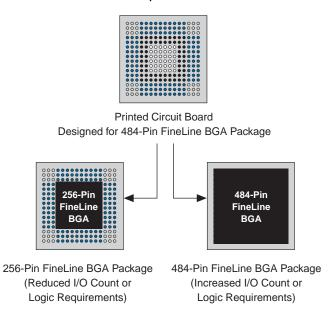
Table 10 shows the ACEX 1K device/package combinations that support SameFrame pin-outs for ACEX 1K devices. All FineLine BGA packages support SameFrame pin-outs, providing the flexibility to migrate not only from device to device within the same package, but also from one package to another. The I/O count will vary from device to device.
