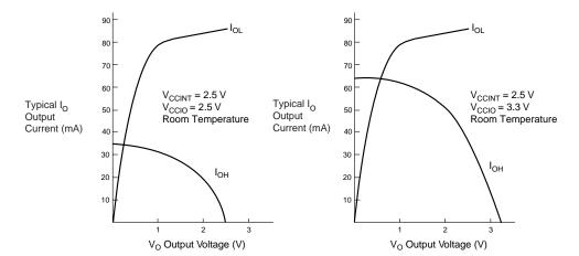
Figure 23. Output Drive Characteristics of ACEX 1K Devices
