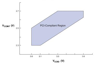
Figure 22. Relationship between V<sub>CCIO</sub> & V<sub>CCINT</sub> for 3.3-V PCI Compliance
