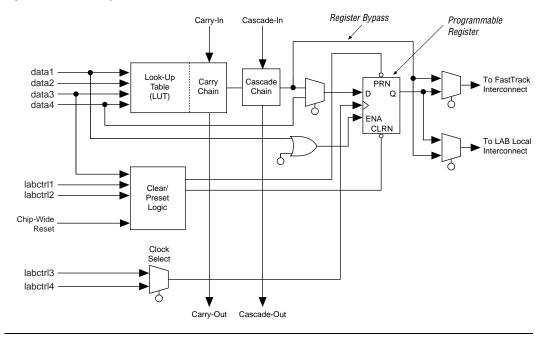
The programmable flipflop in the LE can be configured for D, T, JK, or SR operation. The clock, clear, and preset control signals on the flipflop can be driven by global signals, general-purpose I/O pins, or any internal logic. For combinatorial functions, the flipflop is bypassed and the LUT's output drives the LE's output.
