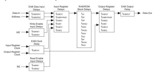
Figure 28. Synchronous Bidirectional Pin External Timing Model
