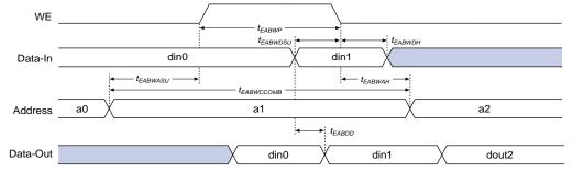
Figure 30. EAB Synchronous Timing Waveforms
