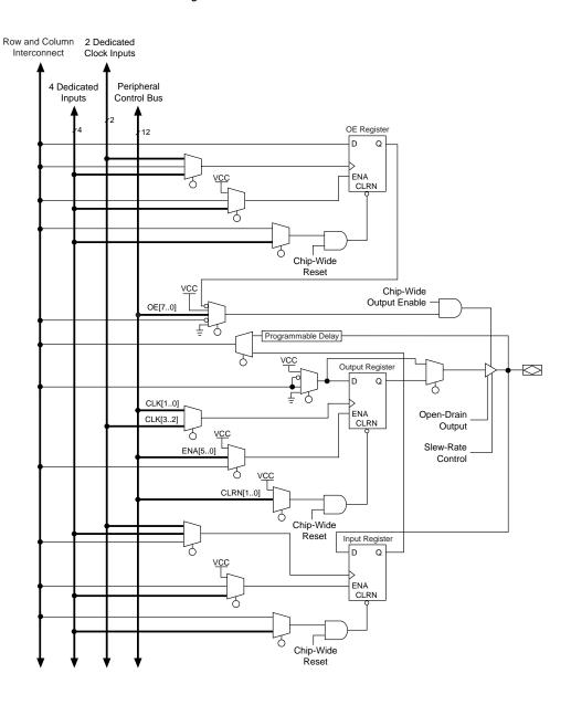
On all ACEX 1K devices, the input path from the I/O pad to the FastTrack Interconnect has a programmable delay element that can be used to guarantee a zero hold time. Depending on the placement of the IOE relative to what it is driving, the designer may choose to turn on the programmable delay to ensure a zero hold time or turn it off to minimize setup time. This feature is used to reduce setup time for complex pin-to-register paths (e.g., PCI designs).
