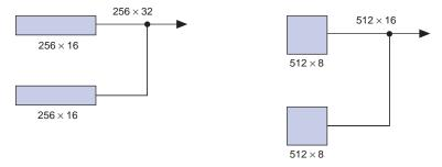
If necessary, all EABs in a device can be cascaded to form a single RAM block. EABs can be cascaded to form RAM blocks of up to 2,048 words without impacting timing. Altera software automatically combines EABs to meet a designer's RAM specifications.
