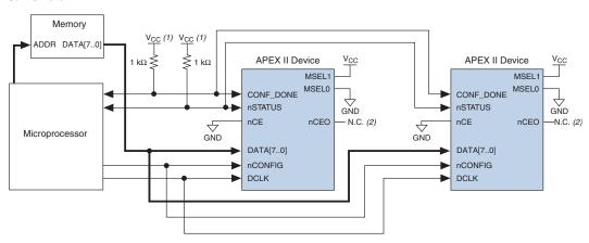
Figure 6–22. Multiple-Device FPP Configuration Using a Microprocessor When Both FPGAs Receive the Same Data
