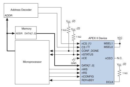
Figure 6–24. Single Device PPA Configuration Using a Microprocessor Note (1)
