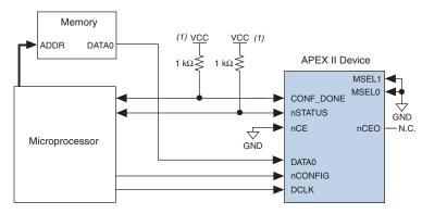
Figure 6-9. Single Device PS Configuration Using a Microprocessor
