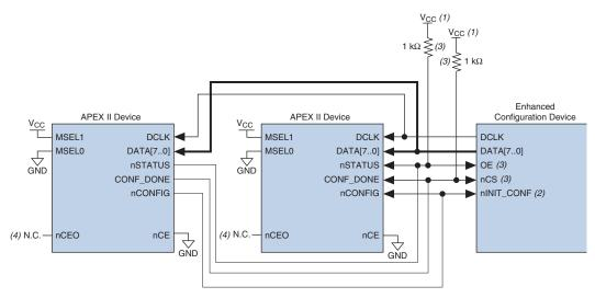
Figure 6–18. Multiple-Device FPP Configuration Using an Enhanced Configuration Device When Both FPGAs Receive the Same Data
