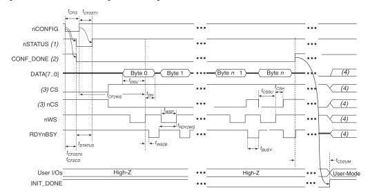
Figure 6-27. APEX II PPA Configuration Timing Waveform
