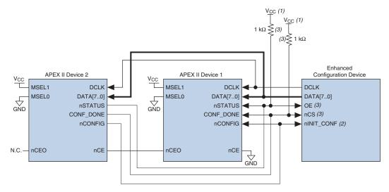
Figure 6-17. Multi-Device FPP Configuration Using an Enhanced Configuration Device
