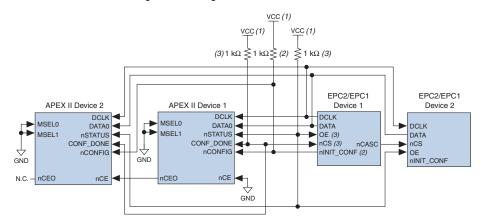
Figure 6–7. Multi-Device PS Configuration Using Cascaded EPC2 or EPC1 Devices
