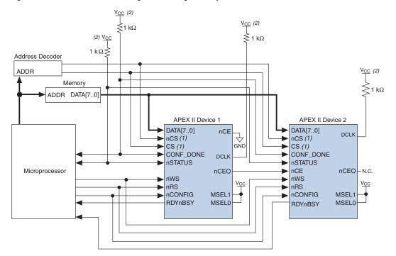
Figure 6–25. Multi-Device PPA Configuration Using a Microprocessor
