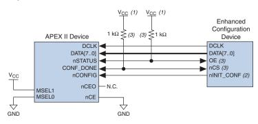
Figure 6–16. Single Device FPP Configuration Using an Enhanced Configuration Device
