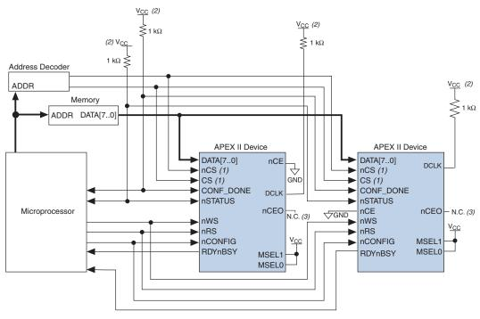
Figure 6–26. Multiple-Device PPA Configuration Using a Microprocessor When Both FPGAs Receive the Same Data
