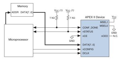
Figure 6–20. Single Device FPP Configuration Using a Microprocessor
