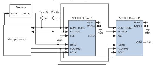
Figure 6–10. Multi-Device PS Configuration Using a Microprocessor
