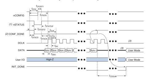
Figure 6-23. APEX II FPP Configuration Using a Microprocessor Timing Waveform
