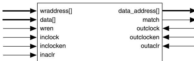
Figure 23. APEX 20KC CAM Block Diagram
