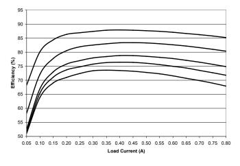
Efficiency Versus Load;  $V_{\text{IN}}$  = 5V,  $V_{\text{OUT}}$  (from top to bottom) 3.3V, 2.5V, 1.8V, 1.5V, 1.2V
