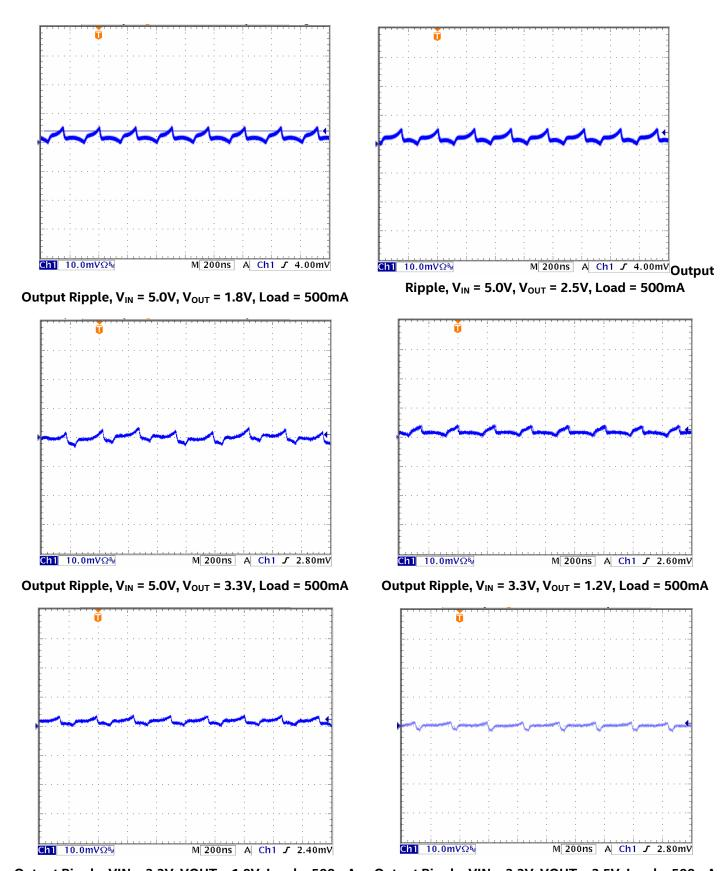
Output Ripple, VIN = 3.3V, VOUT = 1.8V, Load = 500mA Output Ripple, VIN = 3.3V, VOUT = 2.5V, Load = 500mA
