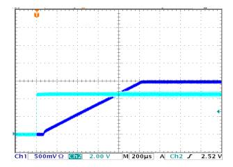
Startup,  $V_{IN} = 3.6V$ ,  $V_{OUT} = 1.5V$ , Load = 500mA.
