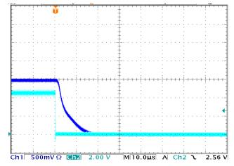
Shutdown, V<sub>IN</sub> = 3.6V, V<sub>OUT</sub> = 1.5V, Load = 500mA.
