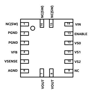
Figure 3. EP5388QI Pin Out Diagram (Top View)
