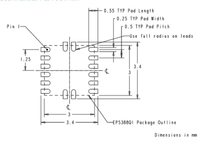
Figure 9: EP5388QI PCB Footprint (Top View)
