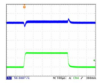
Transient, V<sub>IN</sub> = 5.0V, V<sub>OUT</sub> = 3.3V, Load = 0-800mA
