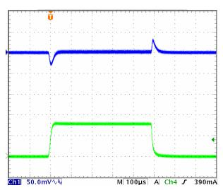
Transient, V<sub>IN</sub> = 3.3V, V<sub>OUT</sub> = 1.2V, Load = 0-800mA
