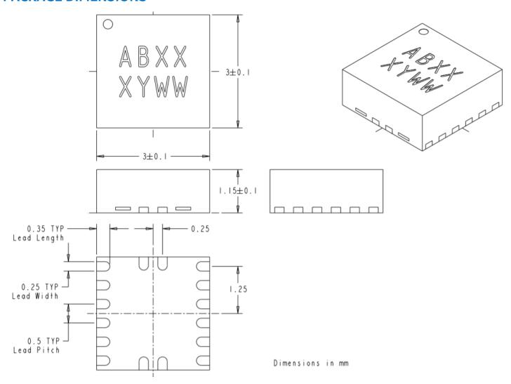
Figure 10: EP5388QI Package Dimensions
