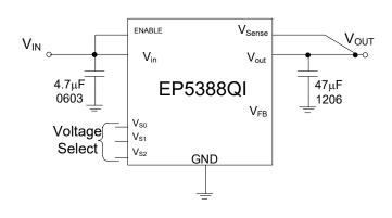
Figure 2. Typical Application Schematic
