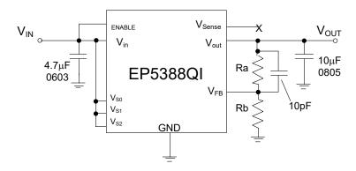
Figure 7. Applications circuit for  $C_{OUT} = 1 \times 10 \mu F 0805$
