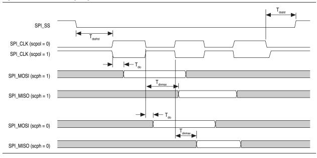
Table 39 lists the SPI slave timing characteristics for Cyclone V devices. The setup and hold times can be used for Texas Instruments SSP mode and National Semiconductor Microwire mode.
