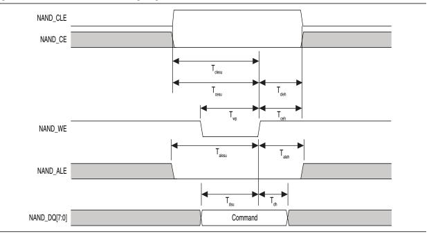
Figure 14 shows the timing diagram for NAND address latch timing characteristics.
