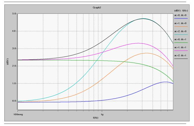
Figure 2 shows the CTLE response at data rates  $\leq$  3.25 Gbps across supported AC gain and DC gain settings for Cyclone V GX, GT, SX, and ST devices.
