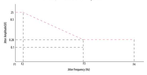
Table 38. LVDS Soft-CDR/DPA Sinusoidal Jitter Mask Values for a Data Rate Equal to 1.6 Gbps
