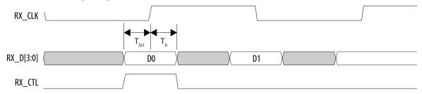
Table 88. Reduced Media Independent Interface (RMII) Clock Timing Requirements for Intel Stratix 10 Devices
