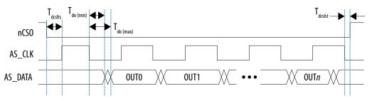
Figure 27. AS Configuration Serial Input Timing Diagram
