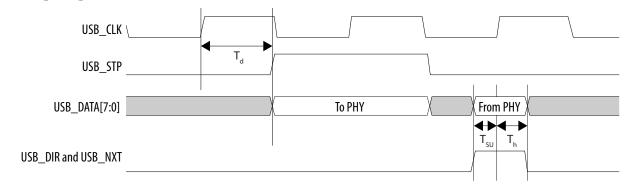
Note: The USB interface supports single data rate (SDR) timing only.
