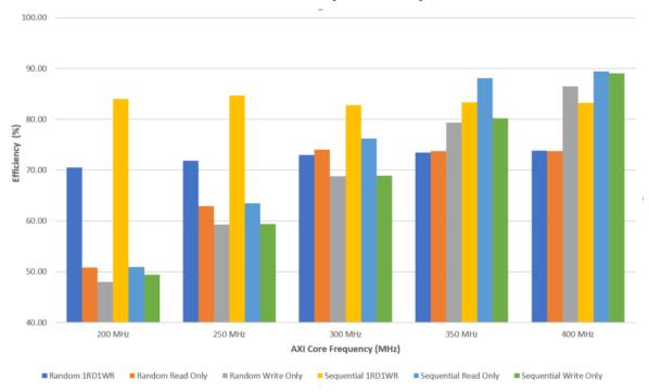
Note: These graphs show the Efficiency information for the HBM2 interface running at 800 MHz in an Intel Stratix 10 MX device with -2 Speed Grade using 64B access, with the re-order buffer turned off and different AXI Transaction IDs enabled.
