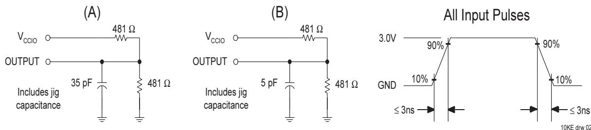
A: Test fixture set-up A is for general testing.
