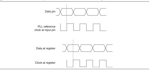
Figure 5-9. Phase Relationship Between Data and Clock in Source-Synchronous Mode
