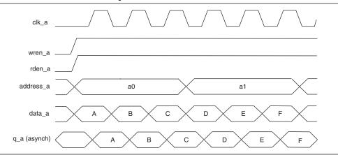
Figure 3-14. Same Port Read-During Write: New Data Mode
