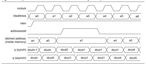
Figure 3–3. Cyclone IV Devices Address Clock Enable During Read Cycle Waveform
