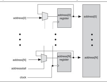
Figure 3–2. Cyclone IV Devices Address Clock Enable Block Diagram
