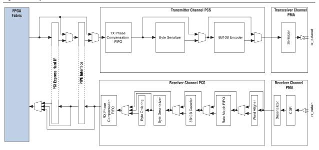
Figure 1–1. Cyclone IV GX Transceiver Channel
