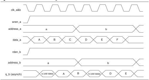
Figure 3–16. Mixed Port Read-During-Write: Old Data Mode
