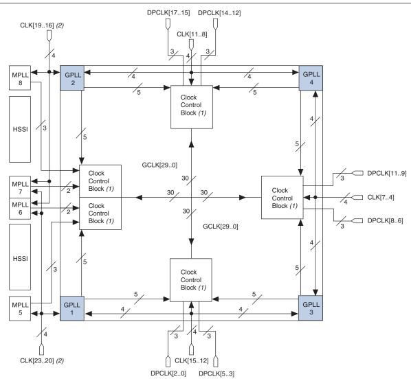
Figure 5–3. Clock Networks and Clock Control Block Locations in EP4CGX50, EP4CGX75, EP4CGX110, and EP4CGX150 Devices
