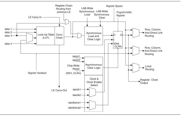
Figure 2-1 shows the LEs for Cyclone IV devices.
