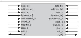
Figure 3–10. Cyclone IV Devices True Dual-Port Memory (Note 1)
