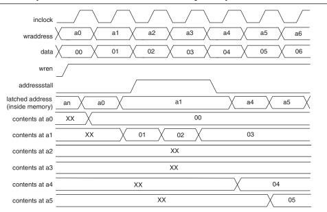
Figure 3–4. Cyclone IV Devices Address Clock Enable During Write Cycle Waveform
