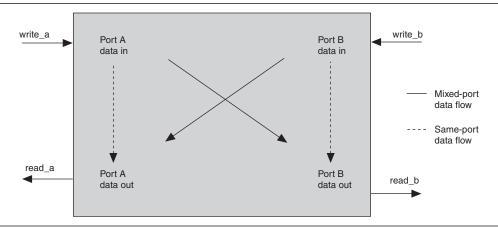
Figure 3–13. Cyclone IV Devices Read-During-Write Data Flow
