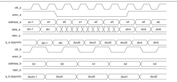
Figure 3–11. Cyclone IV Devices True Dual-Port Timing Waveform
