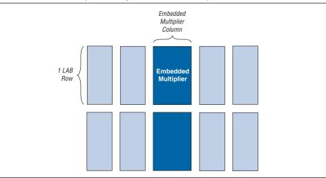
Figure 4-1. Embedded Multipliers Arranged in Columns with Adjacent LABs
