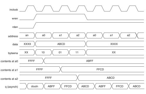
Figure 3–1. Cyclone IV Devices byteena Functional Waveform (Note 1)
